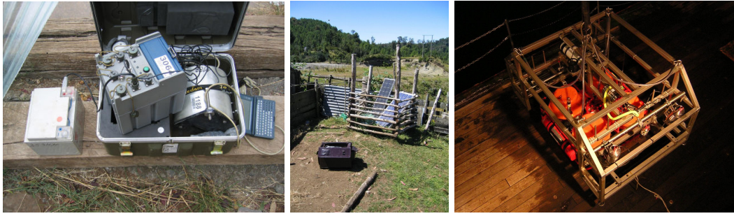
Figure 3.3: Left: EDL station with battery, datalogger and Mark L4-3D seismometer and external service unit. Middle: EDL station deployment with solar panels and additional fence against animals. Right: OBS station.
