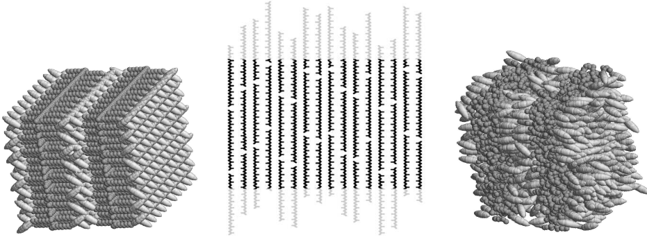
Figure 3. Initial geometrically packed configuration (on the left), backbones interdigitation along the X axis (in the middle) and equilibrated configuration after simulation for 4 ns at atmospheric pressure P = P_{\text{atm}} = 1 atm at T = 500 K (on the right).
