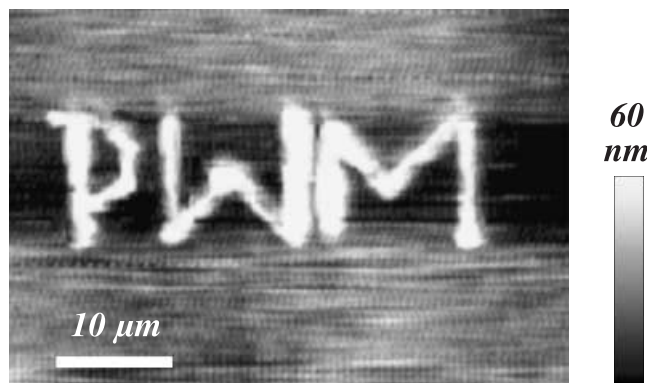
Fig. 8. Example of a non-regular nanostructure in surface topography – PWM (abbreviation from ‘Physik Weicher Materie’) – produced by an illuminated and investigated by a non-illuminated SNOM tip.
