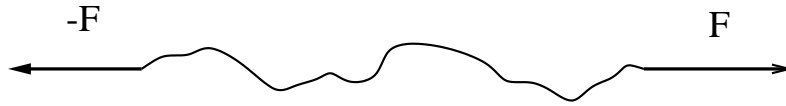
Figure 6.1: Schematic picture of the a membrane under the influence of lateral forces, which leads to a surface tension \Sigma .
